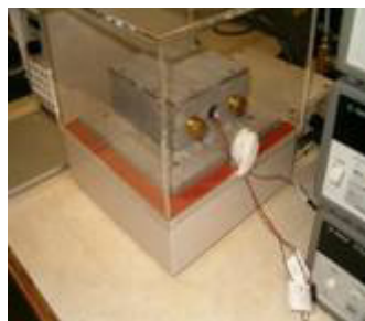
Figure 6. Step-2 DUT temperature sensing probe is placed in the center of the circuit board over thermal compound
