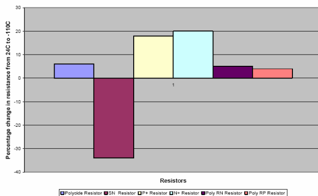
Figure 22. Percentage change in resistance from 24°C to -110°C
