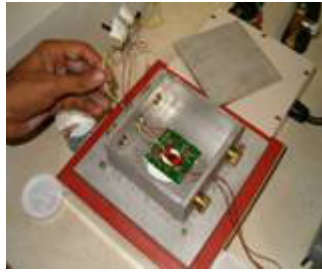
Figure 6. Step-2 DUT temperature sensing probe is placed in the center of the circuit board over thermal compound
