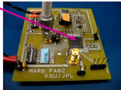
Packaged die on revised PCB
